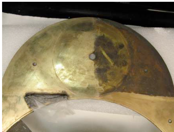
Left: Lunette of faceplate with citrate gel in place. Corrosion has been removed in the bright area at the far right.
