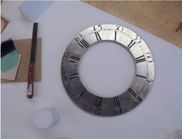
Left: The chapter ring after gilding with palladium leaf
