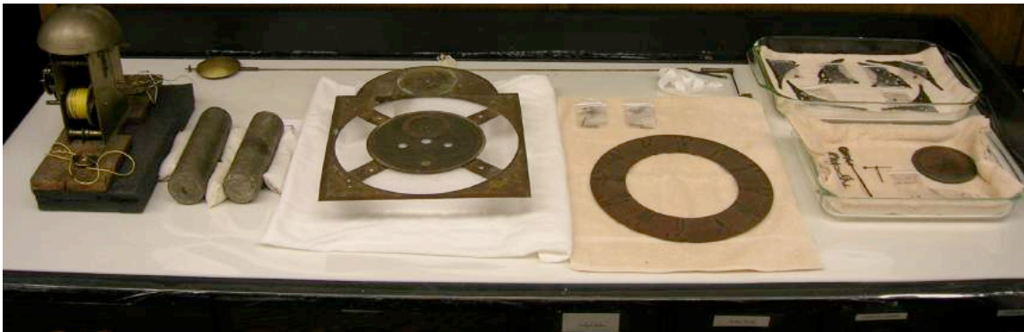
The clock face disassembled into its various components. Note that the seconds ring is still attached, but was later removed.
