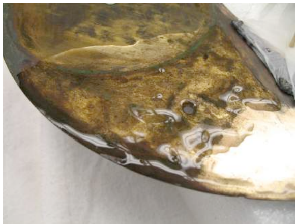
Left: Lunette of faceplate with citrate gel in place. Corrosion has been removed in the bright area at the far right.
