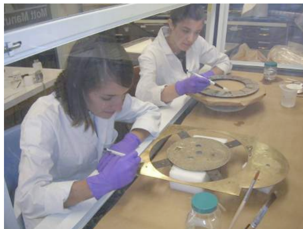
Brush coating the clock face elements with Agateen and Regalrez.
