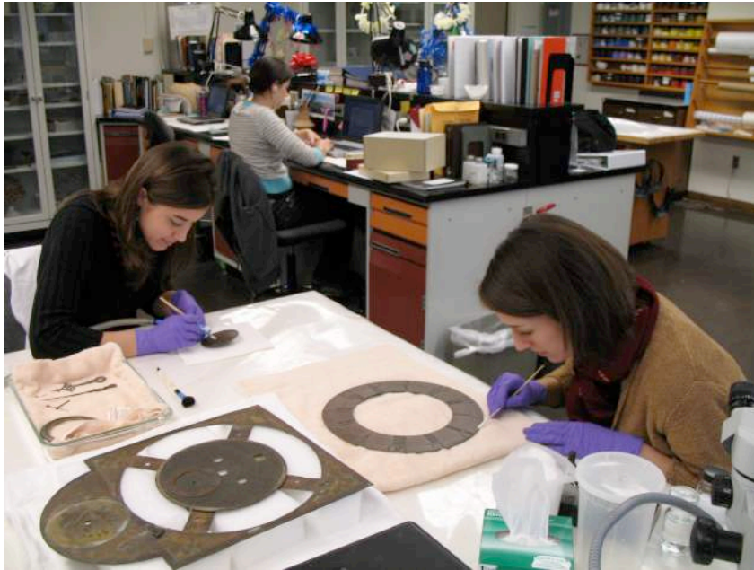
Vacuuming and surface cleaning the clock face post disassembly.
