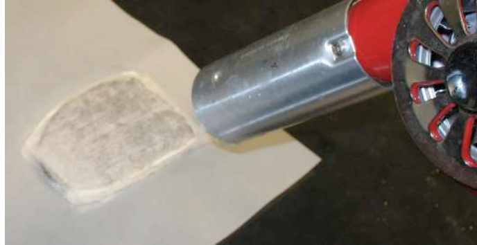
Using heat to melt and adhere BEVA to acrylic paint and paper
