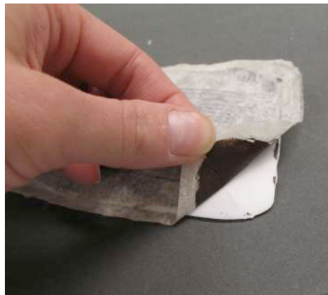
Peeling layers away from mold
